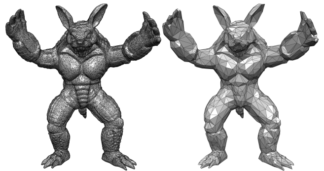
Figure 20: Armadillo. \delta is set to 0.1% and 0.9%. The final vertex count is 26,189 and 1,518. The input model is a surface triangle mesh of the armadillo model with 173k vertices.
