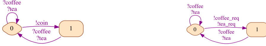
Figure 4: On the left, assumption A_1 , “users shall not insert more than one coin per transaction”. On the right, assumption A_2 , “users shall not press on more than one button per transaction”. In both modal specification the initial state is labeled 0 and has a losange shape.
