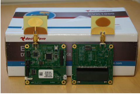
Figure 6. DecaWave's IR-UWB EVK1000 kit with UWB antennas.
