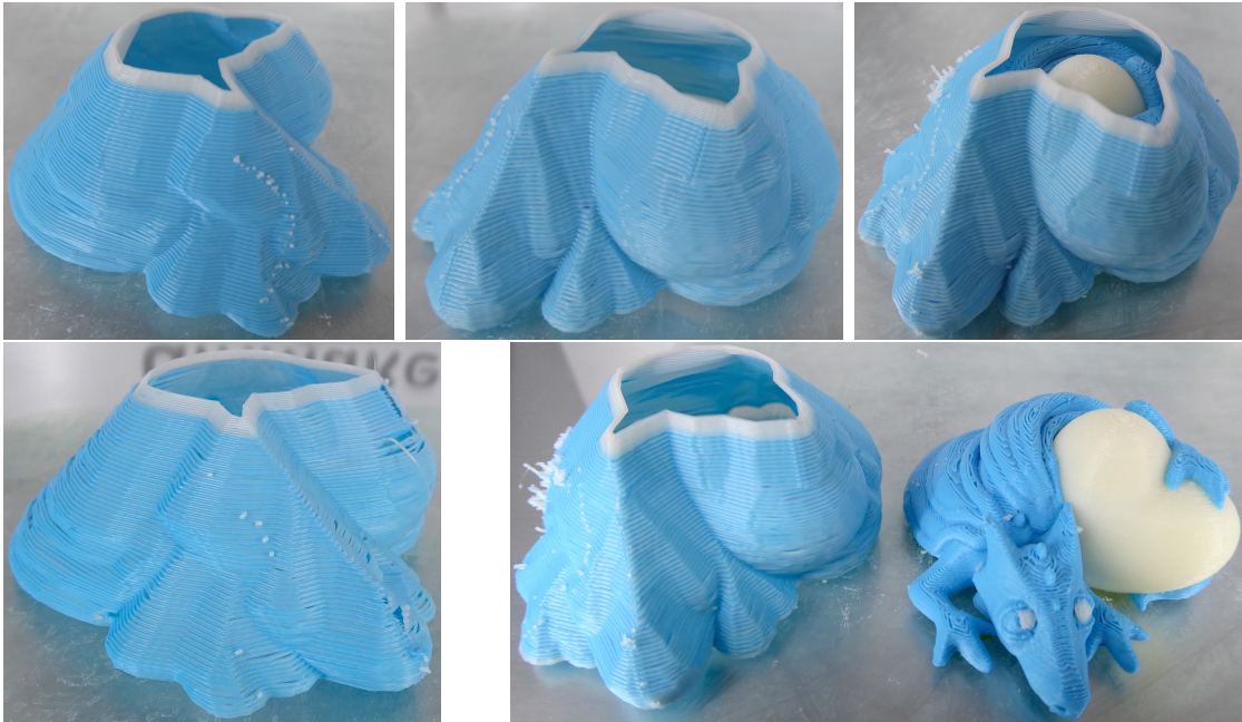
Figure 13: Top. Back and front of a simple enclosure printed alone. The enclosure is two filaments thick and requires no support structure. Each other layer is of a different color. Top right. Same protective enclosure printed with the dual-color dragon model inside. Bottom left. This print is a single filament thick. Bottom right. The dragon has been taken out of its enclosure.
