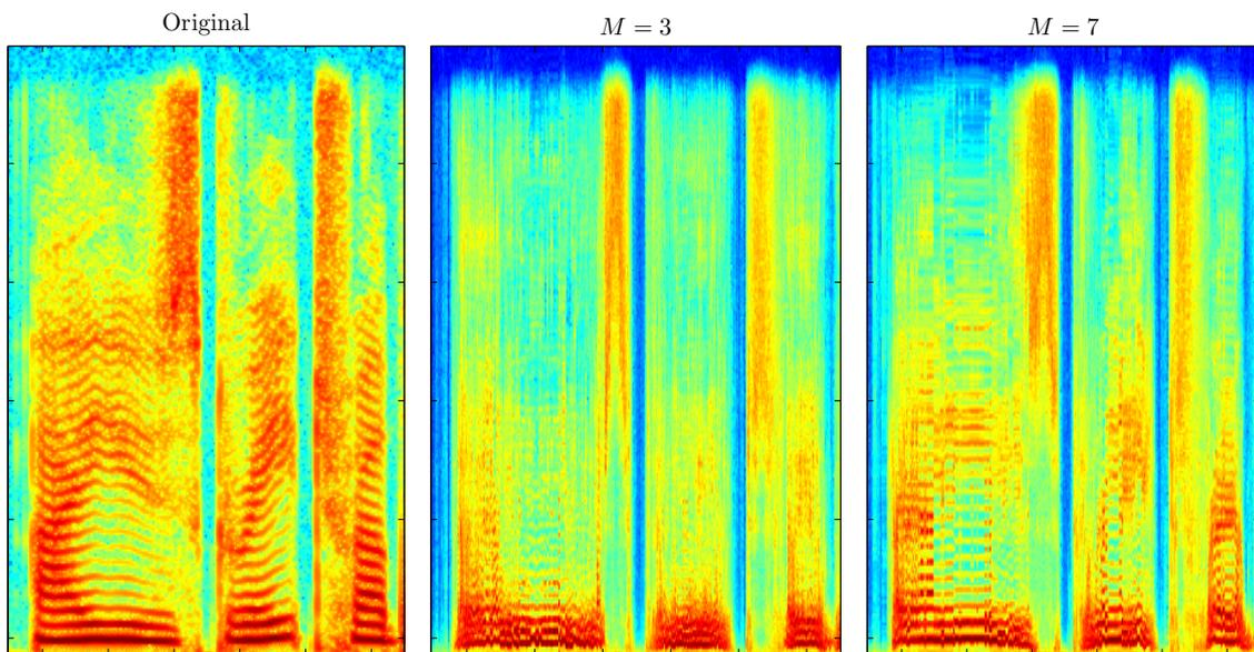
Figure 4.3: Typical reconstruction of a spectrogram using the proposed approach with a development databased composed of  $N = 10^5$  frames, corresponding to 6.6min of continuous audio. Up : original (unknown) test spectrogram to be estimated. Middle : estimate using  $M = 3$  features (zero-crossing rate, onset detection function and frame energy). Down : reconstruction using  $M = 8$  features ( $M = 3$ +spectral centroid, slope, flux and spread).
