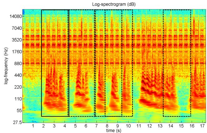
**Fig. 6.** Log-spectrogram of a speech masking a noise. The user selected the region of the first sentence (solid line) and the system identified similar regions where the underlying noise repeats (dashed lines).
