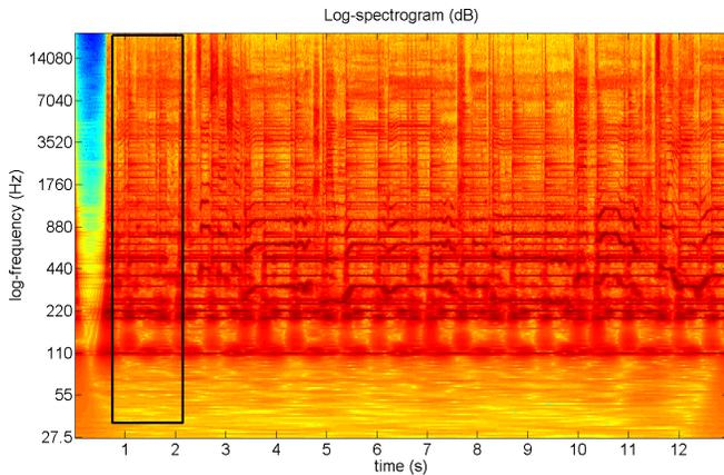
**Fig. 5.** Log-spectrogram of the song with the first measure of the accompaniment recovered. The system averaged the identified regions over their repetitions and filtered out the vocals from the selected region.
