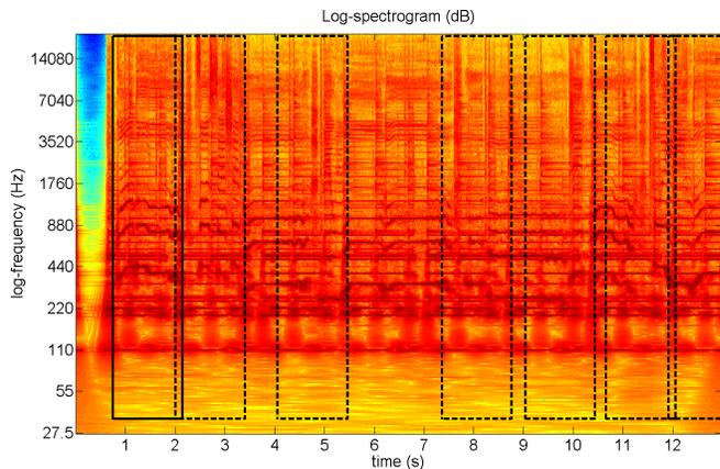
**Fig. 4.** Log-spectrogram of a song with vocals masking an accompaniment. The user selected the region of the first measure (solid line) and the system identified similar regions where the underlying accompaniment repeats (dashed lines).
