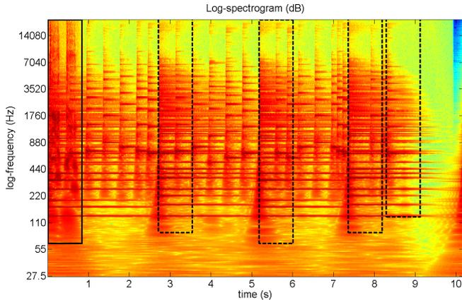
**Fig. 2.** Log-spectrogram of a melody with a cough masking the first note. The user selected the region of the cough (solid line) and the system identified similar regions where the underlying note repeats (dashed lines).
