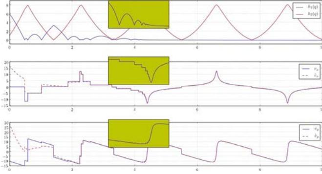
Fig. 4. Velocity estimation error profile for system in Fig. 1(b). The top plot shows the evolution of two gap functions  $h_1(q)$  and  $h_2(q)$  with time. The middle and bottom plot show the velocity components  $v_x$  and  $v_y$ , along with their estimates, respectively. The boxes in the center of these plots provides a magnified image of the quantity of interest around the accumulation point  $t = 4.5$  s.
