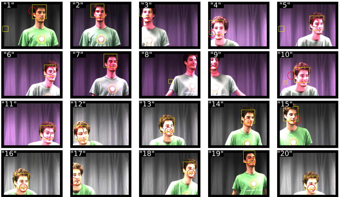
Fig. 4. The moving-speaker scenario. The person is static while he pronounces a number (written in white) and he moves between two numbers. The red circles show the position found with our method. The yellow squares correspond to faces detected with [21]. The full video is available in supplementary materials.
