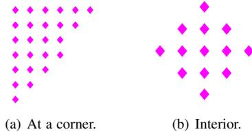
Fig. 4. Pictorial description of the optimal shapes [25]; triangle-like in 4(a) and diamond in 4(b).
