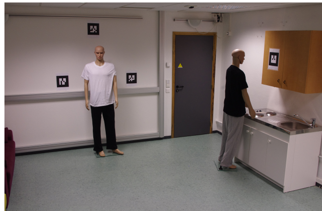
Fig. 2. View of the experimental room. The room is designed to simulate a real living apartment. Some augmented reality tags have been placed around the two dummies.
