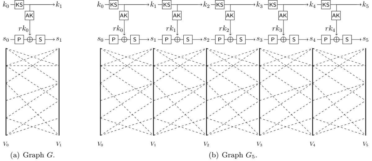
**Figure 3:** Examples of simplified versions of the two graphs  $G$  and  $G_5$ . Variables  $s_i$  and  $k_i$  represent the current internal permutation/key state respectively, while  $rk_i$  stands for the subkey generated during the round.
