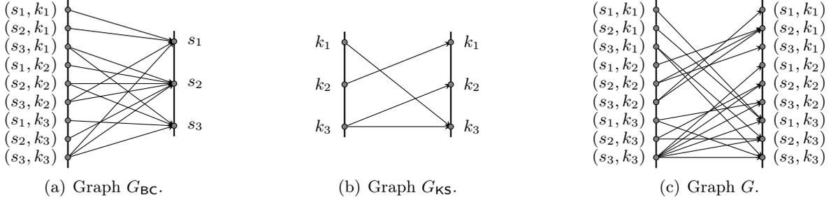
**Figure 4:** Example of graph product to build  $G$ , with three possible internal states  $s_1, s_2, s_3$  and three possible key states  $k_1, k_2, k_3$ , where  $(s_i, k_j)$  represents a node. An edge  $(s_i, k_j) \rightarrow (s_{i'}, k_{j'})$  exists in  $G$  if and only if  $k_j \rightarrow k_{j'}$  exists in  $G_{\text{KS}}$  and  $(s_i, k_j) \rightarrow s_{i'}$  exists in  $G_{\text{BC}}$ .
