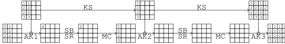
**Figure 12:** The best differential characteristic on two rounds of AES-128, which has a probability  $p = 2^{-6}$ . The vector of differences can take as many as  $2^8$  values, and for instance:  $(1, \dots, 5) = (0 \times 1C, 0 \times 0E, 0 \times 12, 0 \times 01, 0 \times 1D)$ .
