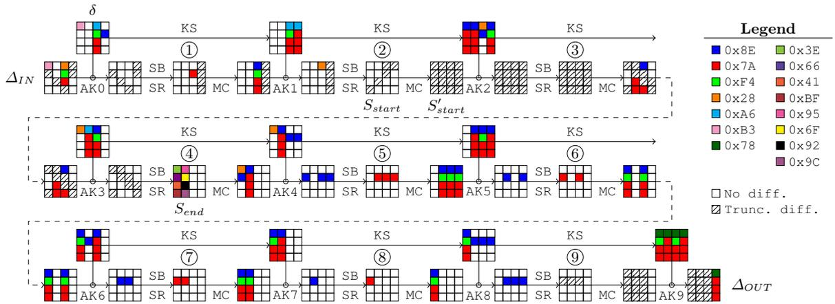
**Figure 6:** Differential characteristic of 9-round AES-128 used in the distinguisher. The colors map to actual values for the differences, whereas hatched bytes are truncated differences and white ones are inactive.
