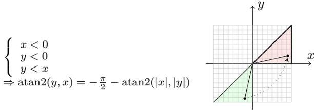
Fig. 2. One case of symmetry-based range reduction. The 7 other cases are similar.
