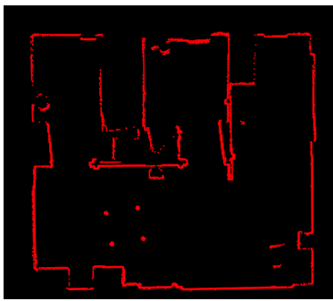
Fig. 9. The superposition of a 3D model (only ground and walls displayed in red) with the map obtained by the SLAM.
