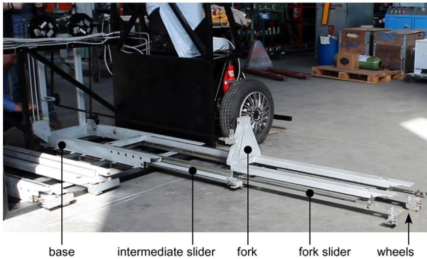
The packaging of this assembly was especially complex due to the small section available for each fork to insert in the slot of the pallet (220 × 90 mm).
