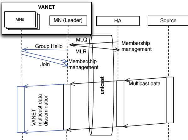
Fig. 2. Extended multicast mobility management for MIPv6.
