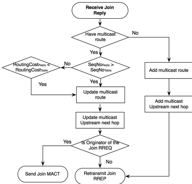
Fig. 3. Join RREP Reception process in MAODV.
