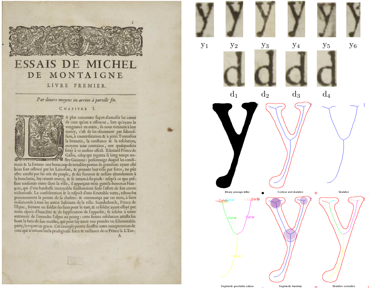
Figure 6. Page from "Essays" by M. de Montaigne, in a 1635 edition 3 from which all instances of printed characters are extracted and clustered by shape. For each cluster, a high resolution average shape is computed, from which further typographically significant measures, related to those in Fig. 4, are derived.
