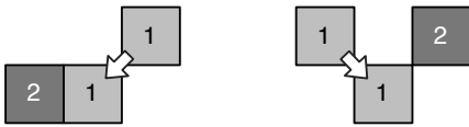
Fig. 2. Minimal 8-connected basic patterns generating temporary labels: stair (left) and concavity (right)
