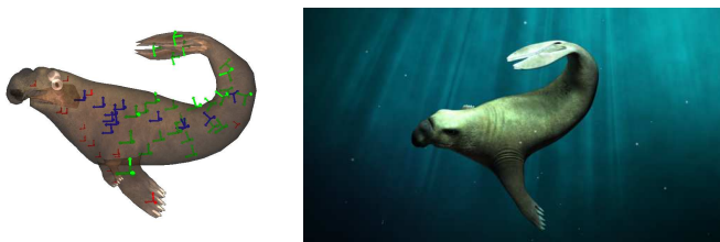
Figure 10: 40 adaptive, elastic frames (green: active, red: passive) adding secondary motion on a (deliberately short) kinematic skeleton corresponding to 12 (blue) frames.
