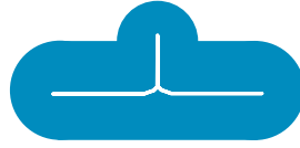
Fig. 7 The medial axis (in white) for a shape (in blue). The junction in the medial axis indicates a branching, which is a criteria for identifying shape features.
