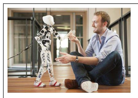
The design of humanoid robots for rich, safe interactions with everyday environments and humans requires techniques for online learning of sensorimotor and social control skills. The opensource 3D-printed humanoid robot Poppy shown here allows systematic experimentation in the integration of such learning methods with adequately designed morphologies (http://www.poppy-project.org; photo Inria/H. Raguet).
