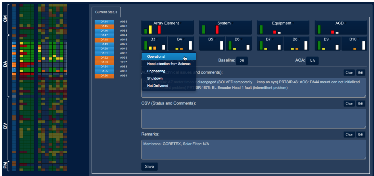
Figure 10. Setting receiver B3 to Operational for antennas DA44 to DA56 with a single edit operation. The small bar charts inside the buttons indicate the distribution of statuses for the corresponding element over the selection of antennas.
