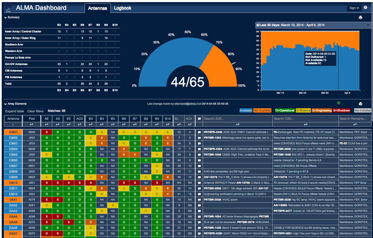
Figure 1. Dashboard main page, giving an overview of antenna availability in the upper part (Summary), and a breakdown of the primary components' operational status for each antenna (Array Elements).
