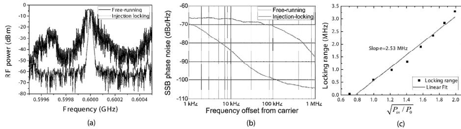
**Fig. 4.** (a) RTD-OEO free-running oscillation and locking to an 8 mW continuous wave optical signal modulated by an RF signal with 0.6 GHz and 500 mV amplitude. (b) Single Side Band phase noise measurements as function of the frequency offset. (c) Locking range as a function of the square root of the injection RF power  $P_{in}$ .
