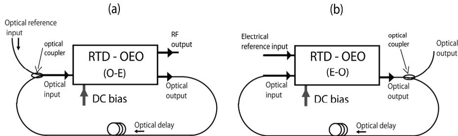
**Fig. 2.** Self-phase locking in (a) optical-to-electrical (O-E) and (b) electrical-to-optical (E-O) schemes. In both cases the optical delay also controls the RTD-OEO providing low-noise E/O conversions.
