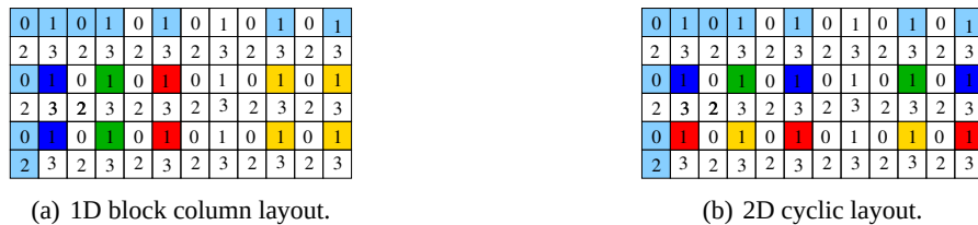
Figure 7: Mapping of threads to supernodal blocks. The light-blue blocks represents the non-empty blocks in the current panel. Four MPI processes are assigned to blocks in a 2 \times 2 grid, where the numbers inside the blocks indicate the process ID. Each MPI process generates four threads; the blue, green, red and yellow blocks are assigned to the first, second, third and fourth thread of process 1, respectively.
