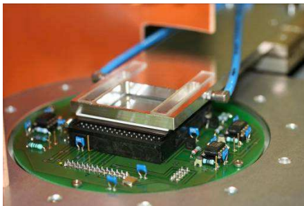
Fig. 5. Assembly of an MLA on a CCD sensor
