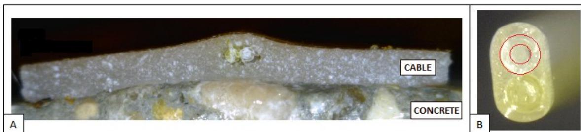
Figure 1: A – View of the cross-section of the cable stuck to the concrete surface. B – Zoom of the cable core, where two fibers and their primary coatings are assembled into a polymer matrix
