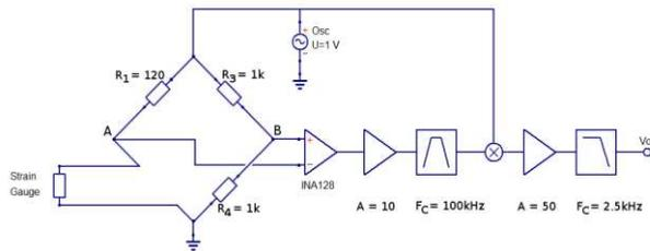
Figure 6 : Circuit schematic for the synchronous detection
