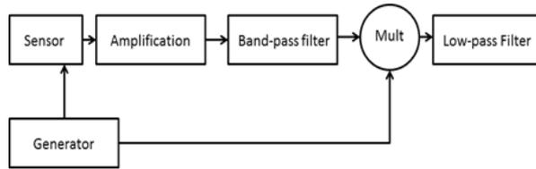
Figure 5 : Schematic of the synchronous detection system
