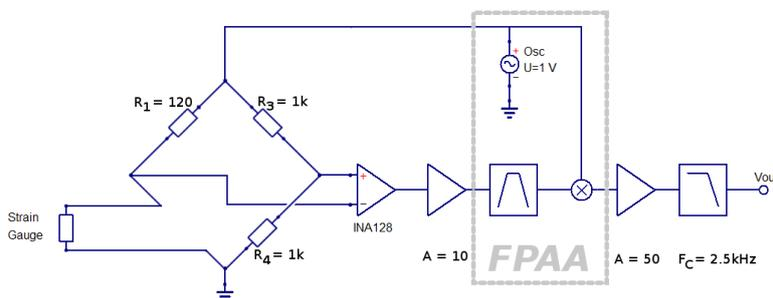
Figure 11 : Synchronous detection integrating the reprogrammable circuit.
