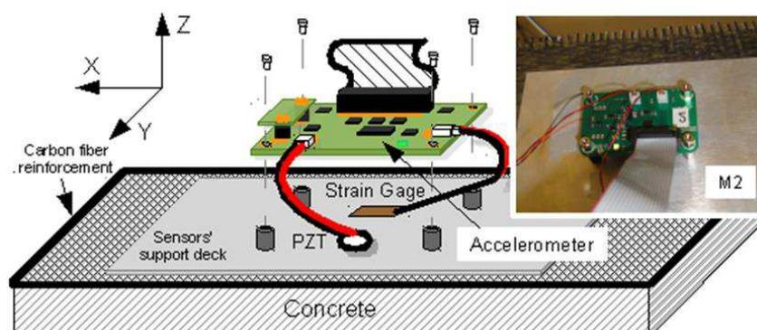
Figure – 3: Detail of the instrumentation architecture of measurement
