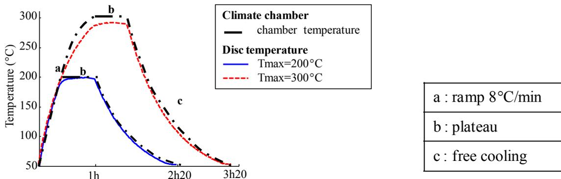
Figure 7 : Thermal cycles
