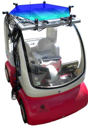
(a) Spherical sensor in ring configuration
