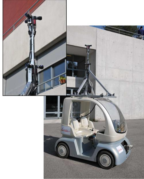
(b) Spherical sensor in vertical configuration
