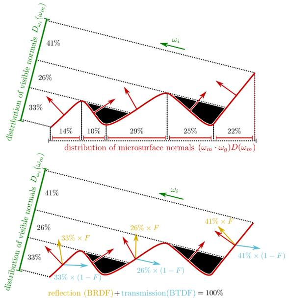
**Figure 3:** The physically-based BSDF model is constructed by applying the operators reflect and transmit on the distribution of visible normals. The ratio of reflection and transmission is given by the Fresnel term  $F$ .
