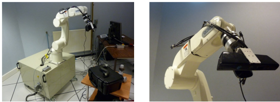
Fig. 3. ADEPT Viper robotic system equipped with a Microsoft Kinect sensor.
