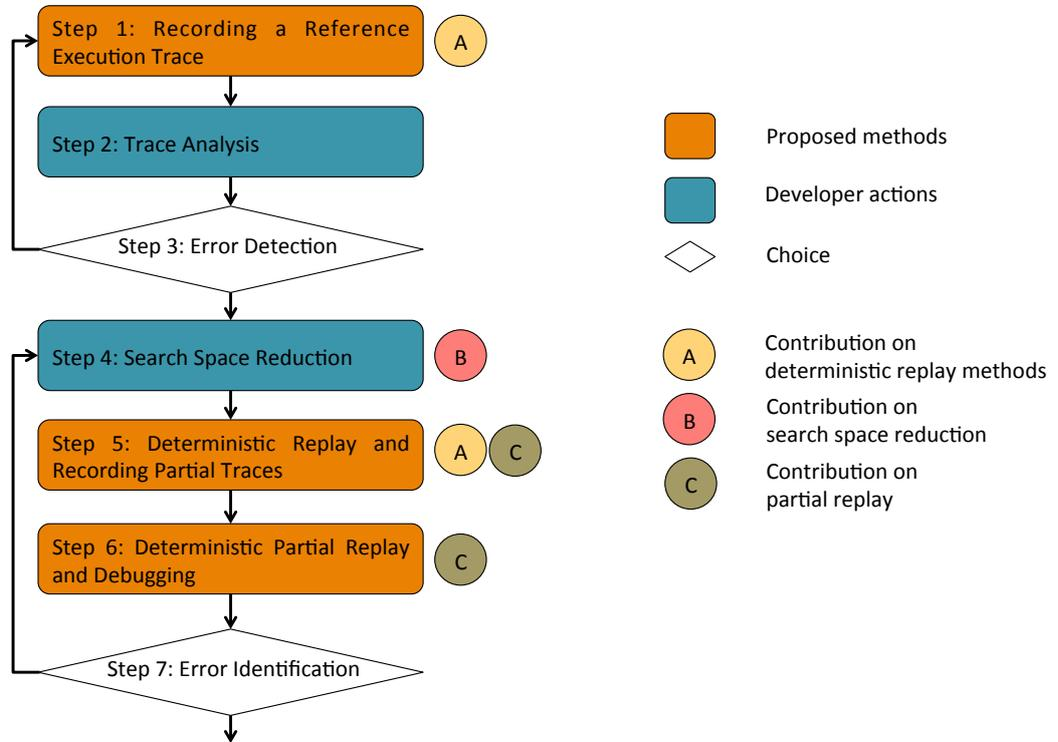
Figure 1: Debugging Cycle
