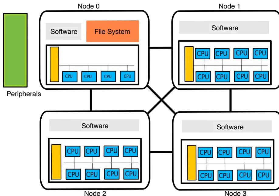
Figure 23: MPSoC Architecture
