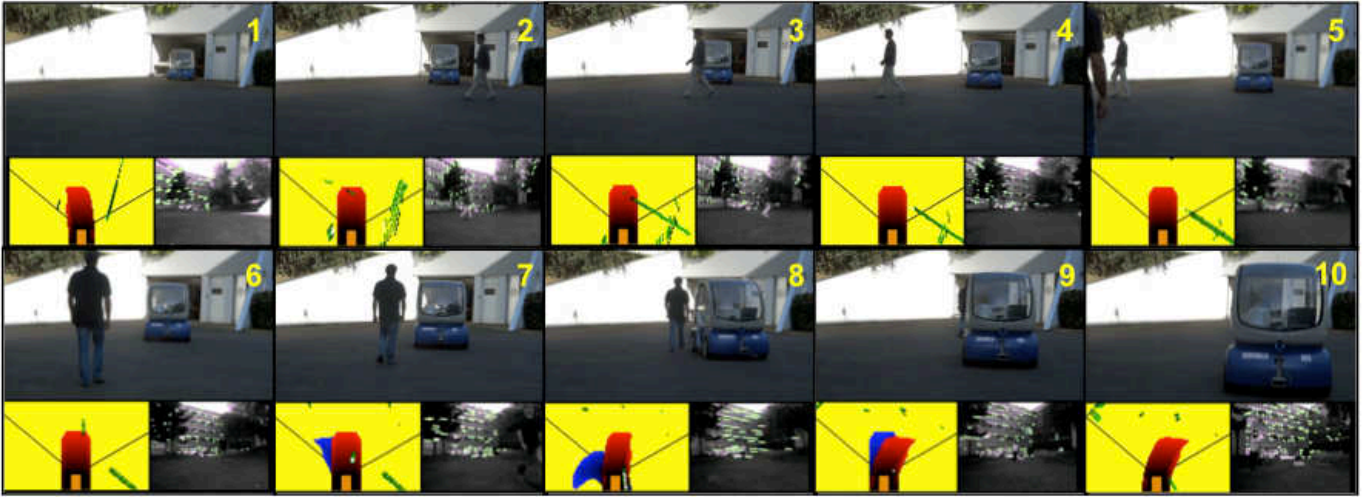
Fig. 3. Ten relevant iterations of the experiment with two crossing pedestrians. For each iteration, we show the occupancy grid (left) and current image (right). In the occupancy grid, the dangerous cell sets associated with the visual tentacle and to the best tentacle (when different) are shown, and two black segments indicate the lidar amplitude. Only cells that we predict to be occupied in the next T s have been drawn in the grid. The segments link the current and next key image points.
