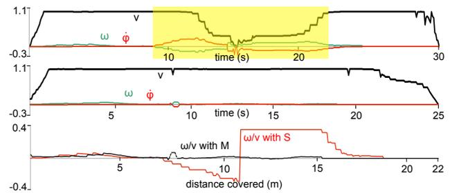
Fig. 5. Single pedestrian experiment. Top and center, respectively: control inputs using S and M, with  $v$  ( $\text{ms}^{-1}$ ),  $\omega$  ( $\text{rads}^{-1}$ ),  $\dot{\varphi}$  ( $\text{rads}^{-1}$ ), and iterations with strong  $H$  highlighted. Bottom: applied curvature  $\omega/v$  (in  $\text{m}^{-1}$ ) using S and M.
