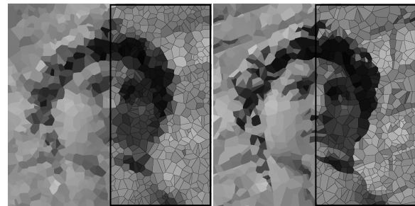
Figure 7: Comparison between a random sampling (left) of an image and our result (right), both using 1000 samples. Objective function values are 0.09 for the random sampling and 0.02 for the optimized one.
