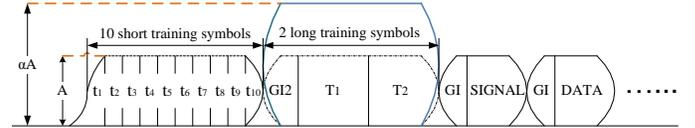
Fig. 2. Structure of the redesigned data packet
