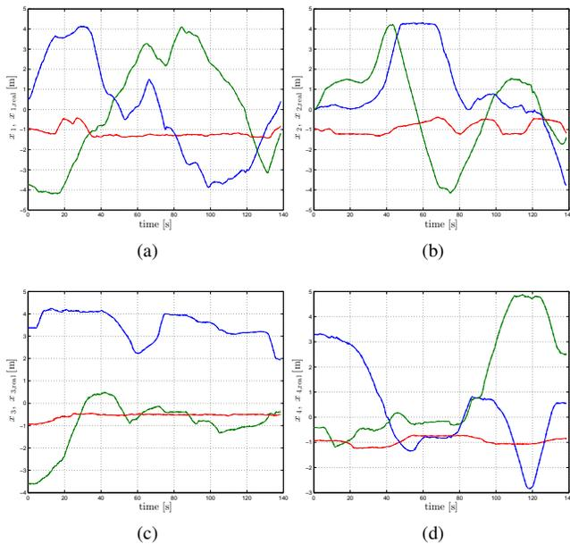
Fig. 21: Results of the experiment: superimposition of  $x_i(t)$  (agent position — solid lines) and  $x_{i,\text{real}}(t)$  (actual quadrotor position — dashed lines) for the 4 quadrotors UAVs used in the experiments. The behaviors of  $x_i(t)$  and  $x_{i,\text{real}}(t)$  are basically coincident, thus showing a very good performance for the quadrotors in tracking the agent motion (4).
