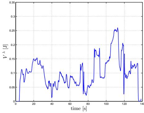
Fig. 15: Results of the experiment: behavior of the Generalized Connectivity Potential  $V^\lambda(\lambda_2(t))$  evaluated on the actual ‘ground truth’ value  $\lambda_2(t)$ . Boundedness of  $V^\lambda(\lambda_2(t))$  confirms that  $\lambda_2(t) > \lambda_2^{\min} > 0$  during the robot motion and, equivalently, that the requirements R1–R3 were always satisfied.
