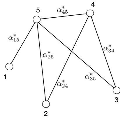
Fig. 6: An illustrative example of the use of the weights  $\alpha_{ij}^*$  in a Graph  $\mathcal{G}$  with  $N = 5$  agents and with the edges representing the sensing-neighbor condition of Definition 1 (sets  $\mathcal{S}_i$ ).
