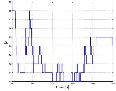
Fig. 14: Results of the HHL simulation: number of edges  $|\mathcal{E}(t)|$  of the interaction graph  $\mathcal{G}(t)$  during the robot motion. One can note how  $|\mathcal{E}(t)|$  changes over time, ranging from 19 to 10, as a consequence of the time-varying nature of the interaction graph  $\mathcal{G}(t)$ .
