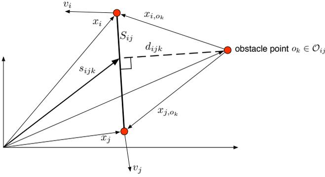
Fig. 2: Illustration of several quantities of interest relative to a pair of agents  $i$  and  $j$ . The agent positions  $x_i$  and  $x_j$ , and their velocities  $v_i$  and  $v_j$ . The segment  $S_{ij}$  (line-of-sight) joining agents  $i$  and  $j$ . An obstacle point  $o_k$  and the corresponding closest point  $s_{ij k}$  on the segment itself. The segment-obstacle distance  $d_{ij k}$ .
