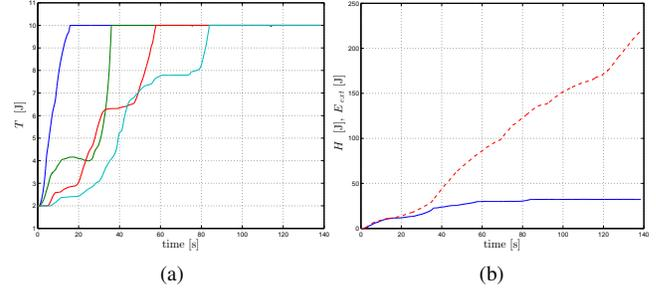
Fig. 17: Results of the experiment. (a): evolution over time of the  $N$  Tank energies  $T_i(t)$  which, after reaching the maximum value  $T_{\max}$ , never discharge. This shows again how implementation of  $\hat{F}_i^\lambda$  was complying with the group passivity condition. (b): behavior of  $E_{\text{in}}(t)$  (blue solid line) and  $E_{\text{ext}}(t)$  (red dashed line). As expected from (39), it is again  $E_{\text{in}}(t) \leq E_{\text{ext}}(t)$ .
