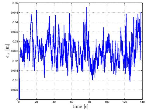
Fig. 22: Results of the experiment: time evolution of the average tracking error  $e_x(t)$  defined in (43) and meant to quantify the accuracy for the UAVs in tracking their desired trajectories in space.
