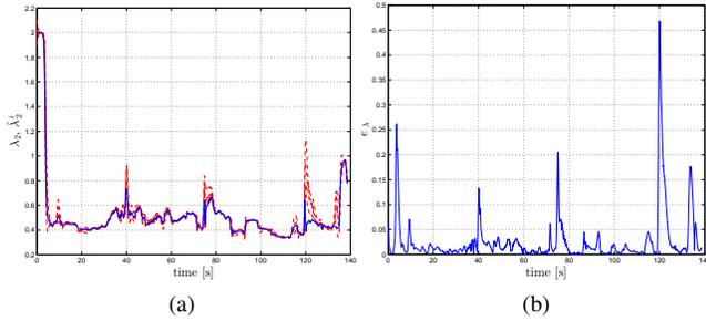
Fig. 16: Results of the experiment. (a): behavior of the ground truth value  $\lambda_2(t)$  (solid blue line) vs. its  $N$  estimates  $\hat{\lambda}_2^i(t)$  (dashed red lines). Similarly to before, the  $N$  estimates are in good agreement with the actual value  $\lambda_2(t)$ . (b): behavior of the estimation error  $e_\lambda(t)$  over time.
