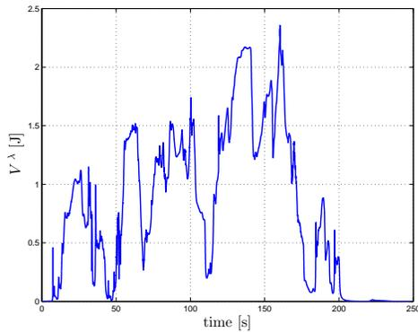
Fig. 9: Results of the HHL simulation: behavior of  $V^\lambda(\lambda_2(t))$  over time. The Generalized Connectivity Potential is evaluated on the real (ground truth) value of  $\lambda_2(t)$  obtained in a independent (and centralized) way w.r.t. the  $N$  estimates  $\hat{\lambda}_2^i(t)$  used by the robots. Boundedness of  $V^\lambda(\lambda_2(t))$  confirms the fulfillment of the requirements R1–R3 embedded in the Generalized Connectivity  $\lambda_2$ .
