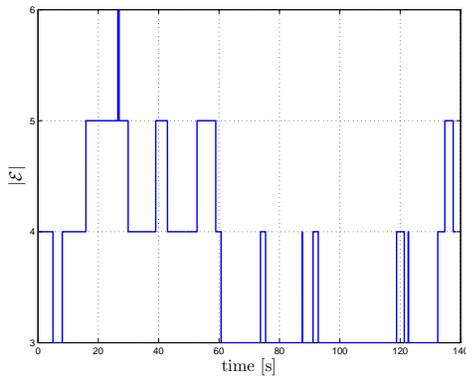
Fig. 20: Results of the experiment: number of edges  $|\mathcal{E}(t)|$  of the interaction graph  $\mathcal{G}(t)$  over time. Note again how (i) the graph topology varies over time, and how (ii) the graph reaches in several phases the ‘sparsest’ possible topology to still ensure connectivity (3 edges for 4 robots).
