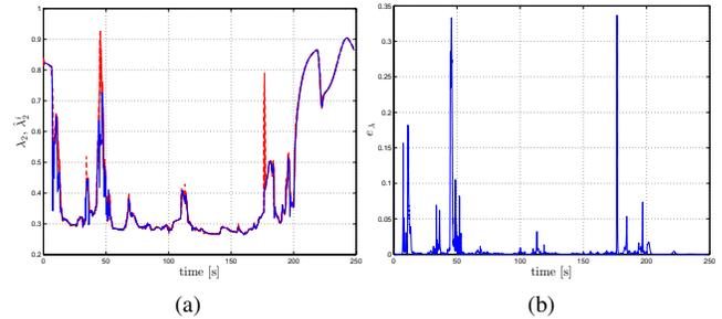
Fig. 10: Results of the HHL simulation. (a): superimposition of  $\lambda_2(t)$  (blue solid line) and the  $N$  estimates  $\hat{\lambda}_2^i(t)$  (red dashed lines). Note how the plots are in very good agreement. (b): behavior of the average estimation error  $e_\lambda(t)$  as per (42).
