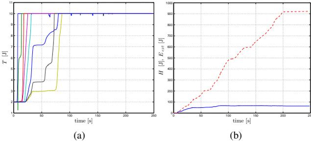
Fig. 13: Results of the HHL simulation. (a): behavior of the  $N$  Tank energies  $T_i(t)$  over time. Note how the Tanks start recharging as the agents move and then almost never discharge, thus confirming that the implementation of the estimated Connectivity force  $\hat{F}_i^\lambda$  by the  $N$  agents did not violate passivity of the group. (b): behavior of  $E_{in}(t)$  (blue solid line) and  $E_{ext}(t)$  (red dashed line). As expected from (39), it is  $E_{in}(t) \leq E_{ext}(t)$ .
