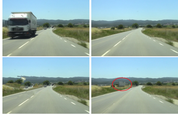
Figure 2. Top : An input frame (left) and the corresponding reference frame (right). Bottom : The results of inpainting (Criminisi et al. [10]) (left) and background estimation (Chen et al. [7]) (right).
