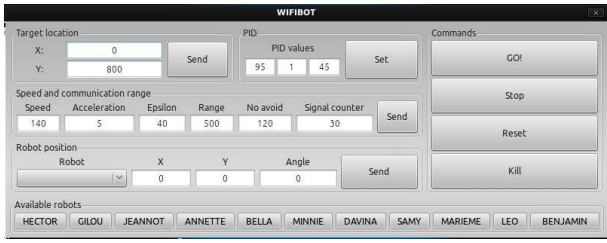
Figure 3: Multi-robot control application.
