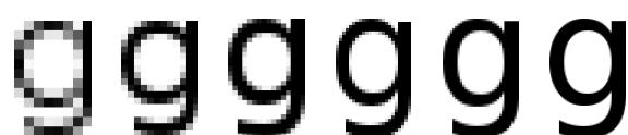
Figure 9. The same glyph rendered at different resolutions (16pt, 24pt, 32pt, 48pt, 64pt, and 128 pt) with greyscale antialiasing.
