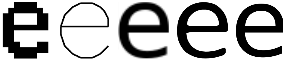
Figure 2. From left to right: bitmap font (GLUT_BITMAP_HELVETICA_12), stroke font (GLUT_STROKE_ROMAN), texture font (Bitstream Vera, 64 points), signed distance field font (Bitstream Vera, 32 points), and vector font (Bitstream Vera).
