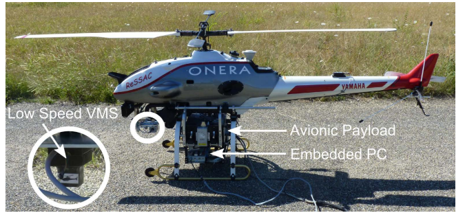
Fig. 6. The ONERA ReSSAC Unmanned Autonomous Helicopter before takeoff, featuring the on-board low-speed VMS mounted at the front end looking downward
