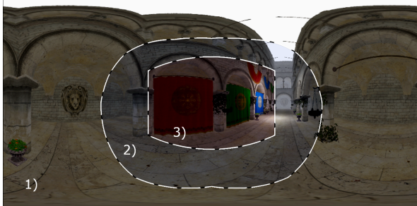
Figure 3: Comparison of the fov provided by 1) equirectangular projection, 2) human natural binocular vision (light blue), 3) classic perspective projection (light red) with 16:9 aspect ratio (75° × 107.5°).
