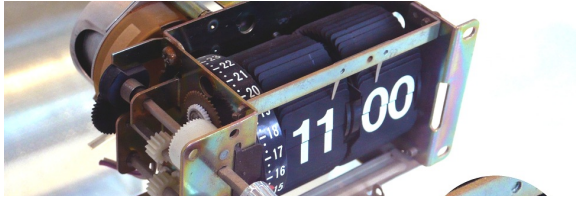
Figure 5: This type of split-flap display is probably best known from airport information panels. By replacing the numbers with a set of material samples, one would obtain a trivial two-pixel BRDF display capable of full 4 \rightarrow 4 interaction, but with 0D parameterization.
