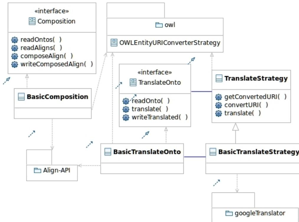
Figure 1: Class diagram for Multi-Align API.
