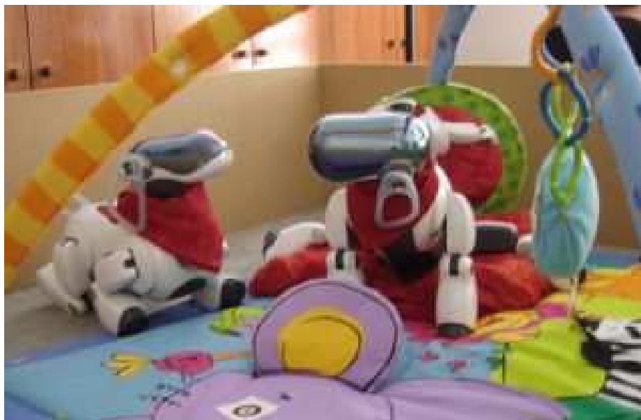
Fig. 1. The Playground Experiment setup involves a physical Sony AIBO robot which is put on a baby play mat with various toys, some of which affording learnable interactions, and an “adult robot” which is pre-programmed to imitate the vocalization of the learning robot when this later robot produces a vocalization while looking in the direction of the adult robot. The learning robot is equipped with a repertoire of innate parameterized sensorimotor primitives, and learns driven by intrinsic motivation how to use and tune them to affect various aspects of its surrounding environment. Complex self-organized developmental trajectories emerge as a result of intrinsically motivated exploration, and the set of acquired skills and affordances increases along with time.
