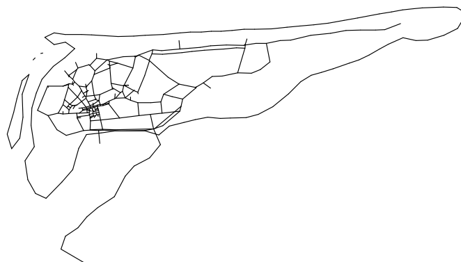
Figure 4. Map from Figure 3 after simplification from 2086 edges to 452 edges using progressive meshes, with intersections and end nodes pinned to their original locations.
