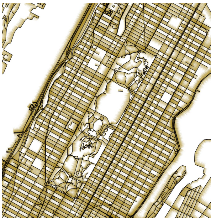
Figure 14. Manhattan with Central Park, simplified with Ramer-Douglas-Peucker to about ½ of the original edge count.
