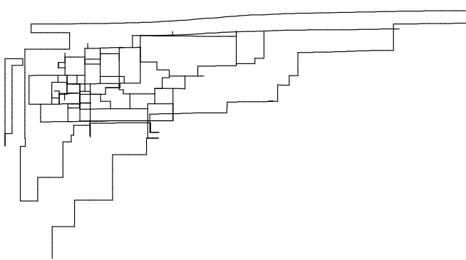
Figure 6. Map from Figure 3 (first simplified without restrictions using progressive meshes to 658 edges), after 555 iterations of the rectangularization technique.
