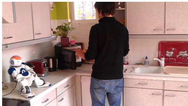
Fig. 1: This figure shows a robot companion, i.e., the humanoid robot NAO, listening to a person involved in an everyday kitchen activity. Using the continuous sound recognition method described in this paper, NAO is able to extract a discrete sequence of isolated sounds and to interpret them in terms of a pre-stored catalogue of auditory events (microwave alarm, open microwave door, close microwave door, toaster, etc.), all in the presence of background noise, competing sound sources, and reverberations. Remark how difficult would be to recognize this human activity using vision.
