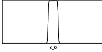
Figure 2: Spreading function \delta^{\mathcal{H}}(x) used to model the hammer string contact. The width of the contact zone is about 2 cm.
