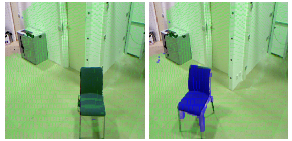
(a) The chair is considered as a static object. (b) The chair has been moved and is considered as a mobile object.
