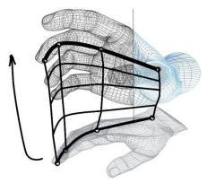
Figure 2. Bézier surface drawn by hand movement.
