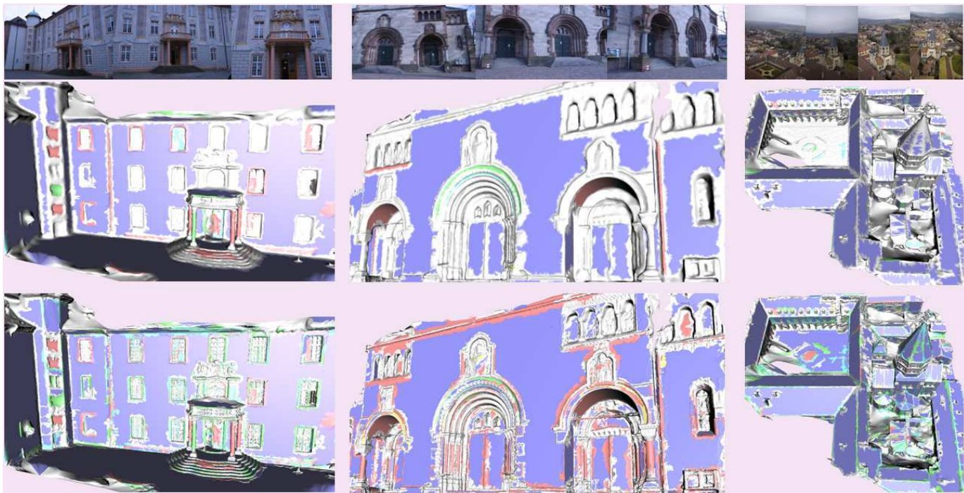
Fig. 10. Facade and roof reconstruction. Top row: some input images. Middle and bottom rows: hybrid models at low and high resolutions. From left to right: Entry-P10, Herz-Jesu-P25 and Church datasets. Color code: see Fig. 7.
